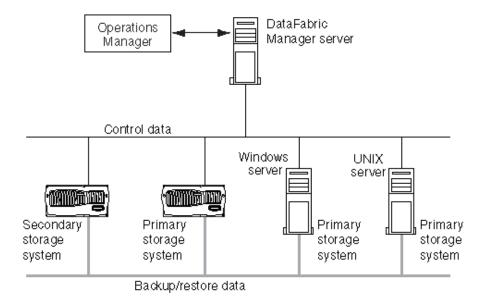
The configuration provides data protection between two storage systems and from a storage system to a UNIX or a Windows storage system.
